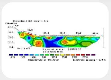
Geophysical tools such as Ground Penetration Radar (GPR), Seismic Refraction, Seismic Reflection, Electrical Imaging etc., can be used for the accurate mapping of the underground infrastructure facilities (Electrical & telecommunication cables, pipelines etc.), soil-rock interface, geological identification of soil, water table mapping, dimension of a sub stratum, elastic properties of the medium, geometry of various layers and other subsurface features.
